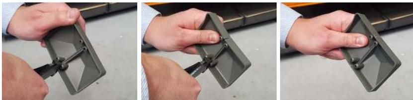
Cut each side of the cap in line with the centre ridge. Use end-nippers – do not use a knife as this is dangerous and difficult to achieve a straight cut. Ensure the 'nose' of the end nippers is pushed all the way in before cutting.
