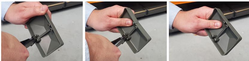
Cut each side of the cap in line with the centre ridge. Use end-nippers – do not use a knife as this is dangerous and difficult to achieve a straight cut.
