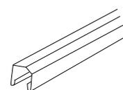
Standard ColourSlat™ panels are 2350mm wide which is also the standard length for Boundaryline rails. The slat length is determined by subtracting 40mm from the distance between your posts; eg. 2350mm panel will require 2310mm slat length.
