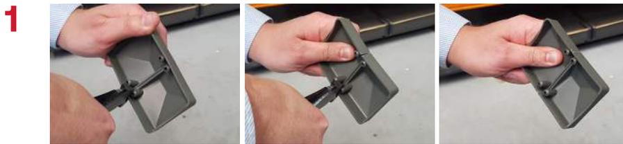
Cut each side of the cap in line with the centre ridge. Use end-nippers – do not use a knife as this is dangerous and difficult to achieve a straight cut.
