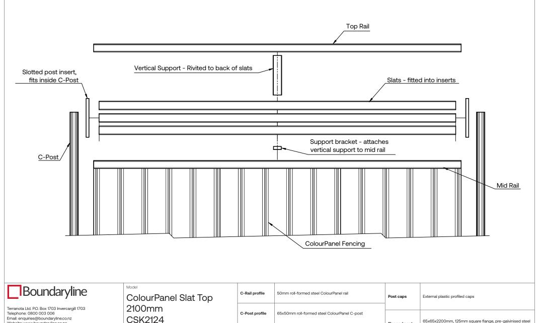
CSK2124 65x65x2200mm, 125mm square flange, pre-galvinised steel Website: www.boundaryline.co.nz Flanged post powdercoated to match, M12 fixings ©Copyright June 2017. All rights reserves to Terranota Ltd Slat profile 55x7.5mm steel slat set at 25mm spacing DO NOT SCALE **Exploded view A4** 2023-03-31 DRAWING 65x65x2800mm pre-galvinised steel powdercoated to In-ground post Weight 2380mm wide x 2100mm high Panel length 2 of 2 Unless otherwise specified, dimensions are in millimetres
